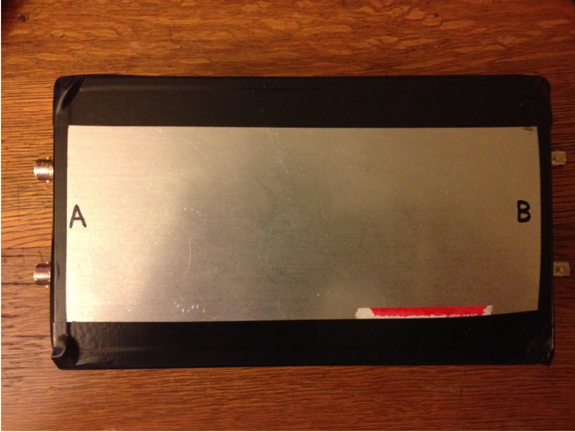
Figure 21. The light-tight aluminum box used for SiPMT experimentation. The box measures 19 \times 11 \times 6 cm and is labeled A and B for the dual ended SiPMT experimentation. Black vinyl electrical tape was used to cover the edges of the lid-box interface to reduce the amount of light leakage into the aluminum box.
