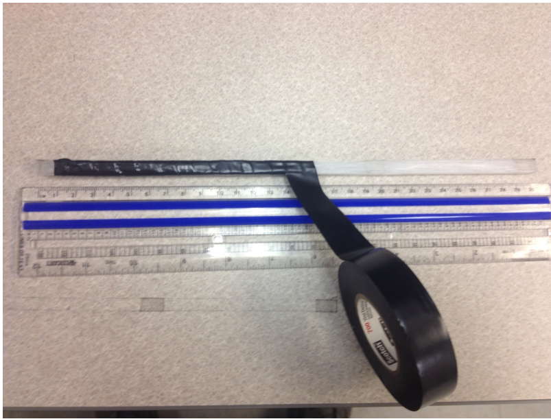
Figure 17. The “z-axis” view of the 14 \times 14 BCF-12 fiber bundle array. The bundle is wrapped in black vinyl electrical tape to help mitigate light leakage out of the bundle. The tape was applied at a approximately a 45 deg angle and three layers were applied.
